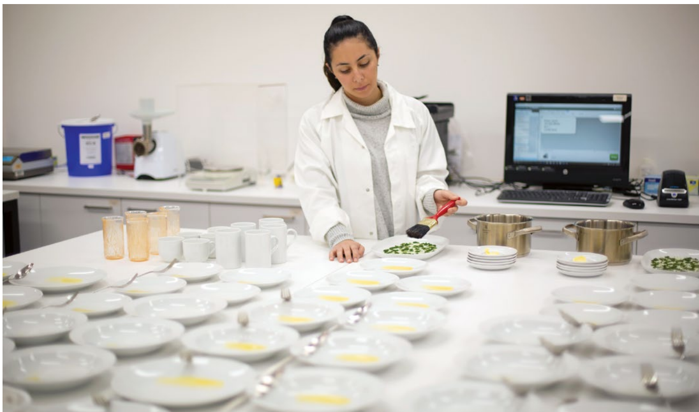
CHOICE expert Rebecca Ciaramidaro does the painstaking job of ‘dirtying’ standardised sets of crockery with different types of food to test dishwashers.
